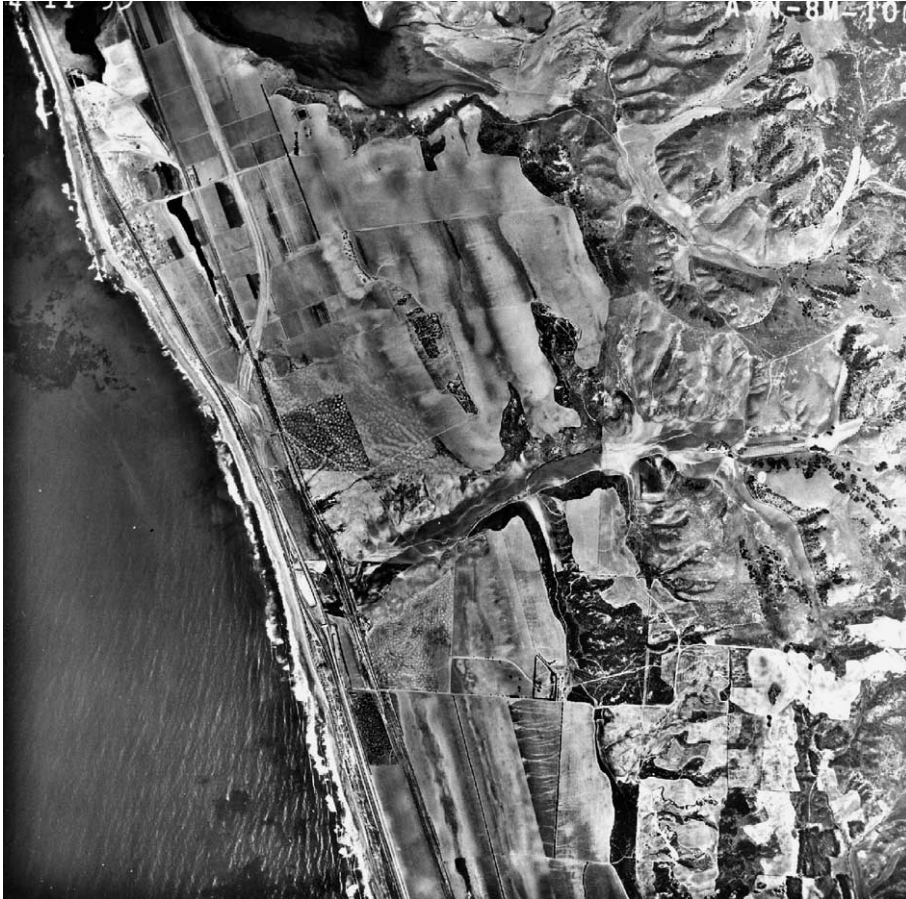
Fig. 5. 1953 vertical aerial view of the coastal lagoons and terraces at Carlsbad, California. The circular features located in the center of the photograph are “mima mounds;” many are now confirmed to be “sand blow” deposits. Thus several lineaments include lateral spread surfaces or fissure fills (photograph from U.S. Department of Agriculture Photograph #AXN-8M-100, taken on 11 April, 1953).
